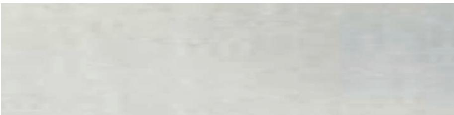
A finer, more random pattern than a number 4 finish. It is used in architectural applications where a lower luster of material is desired, or to contrast with brighter finishes. This finish can be field repaired, however, due to its soft pattern and inherent random design, scratch removal is a timely process. In addition, the original finish may not be retained.
